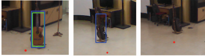
Fig. 12. Results of object detection using HOG-SVM. The red dot is the position localized by RFID, projected in image space. The object detected is bounded by the rectangle (blue, green) from both frontal and side HOG-SVM detectors.
