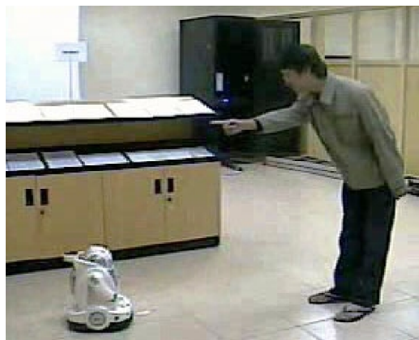
Figure 3: An example of scenario in which a human asks the robot to know more about the abstract of a book to which his hand is pointing. The robot will answer the human by synthetic voice using Vietnamese speech synthesis system.
