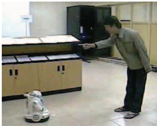
Figure 2. An example of scenario in which a human asks the robot to know more detail about the abstract of a book to which his hand is pointing. The robot answers the human by synthetic voice using Vietnamese speech synthesis system.
