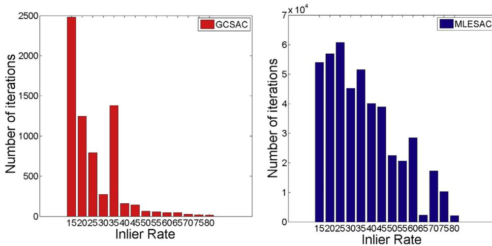
**Fig. 6.** The number of iterations of GCSAC (left side) and MLESAC (right side) for estimating a cylinder from point clouds in the first dataset. The results are given by averaging 50 run times.
