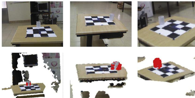
**Fig. 10.** The cup is detected by fitting a cylinder. Top row: The scenes in Dataset 3 captured at different view-points; Bottom row: The results of locating a coffee cup using GCSAC in corresponding point clouds.
