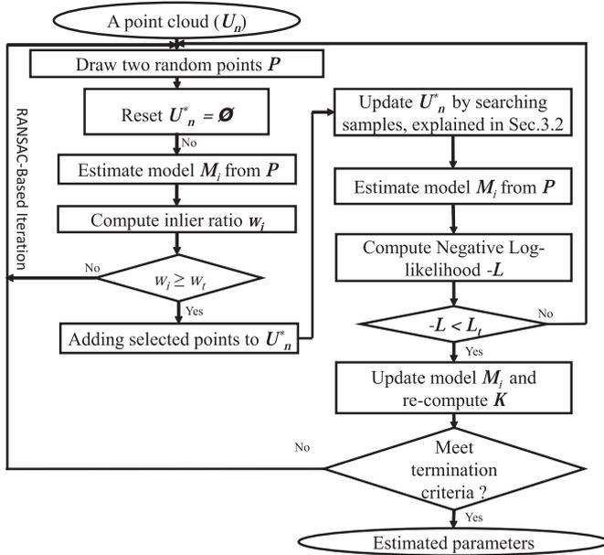
**Fig. 3.** A diagram of the cylindrical object estimation using GCSAC.
