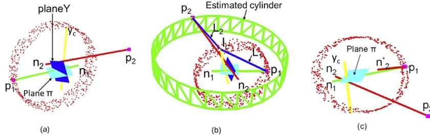
**Fig. 4.** (a) Setting geometrical parameters for estimating a cylindrical object from a point cloud as described in Section 3.2. (b) The estimated cylinder (green one) from an inlier  $p_1$  and an outlier  $p_2$ . As shown, it is an incorrect estimation. (c) Normal vectors  $n_1$  and  $n_2$  on the plane  $\pi$  are specified. (For interpretation of the references to colour in this figure legend, the reader is referred to the web version of this article.)
