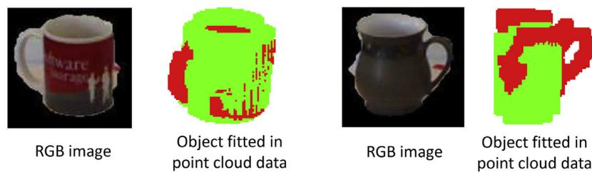
**Fig. 9.** Result of coffee mug fittings. Ground-truth objects are marked as red points; estimated ones are marked as green points. (For interpretation of the references to colour in this figure legend, the reader is referred to the web version of this article.)
