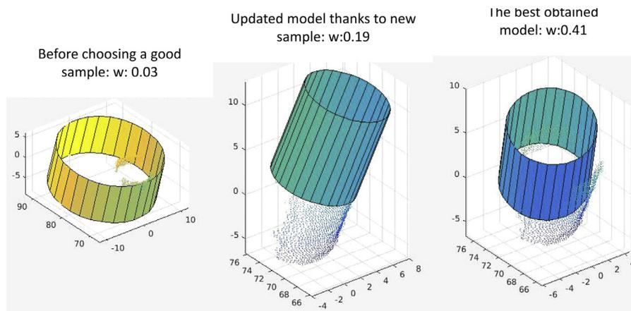
**Fig. 8.** An illustration of GCSAC's at a  $k$ th iteration to estimate a coffee mug in the second dataset. Left: the fitting result with a random MSS. Middle: the fitting result where the random samples are updated due to applying the geometrical constrains. Right: the current best model.
