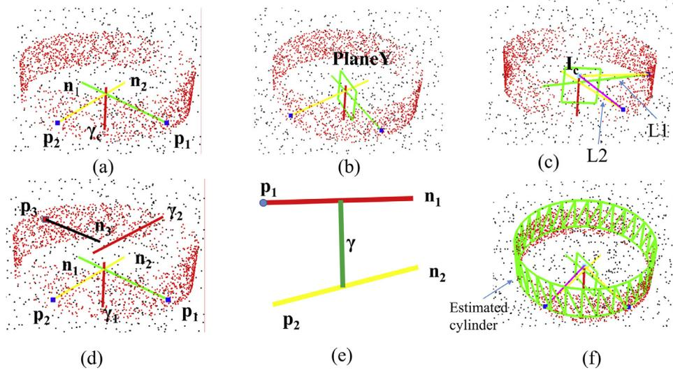
**Fig. 2.** Geometrical parameters of a cylindrical object. (a)–(c) Explanation of the geometrical analysis to estimate a cylindrical object. (d)–(e) Illustration of the geometrical constraints applied in GCSAC. (f) Result of the estimated cylinder from a point cloud. Blue points are outliers, red points are inliers. (For interpretation of the references to colour in this figure legend, the reader is referred to the web version of this article.)
