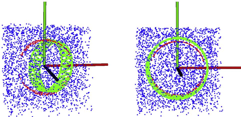
**Fig. 7.** The estimated cylinders (green points) in a point cloud of the first dataset with only 10% inlier. Right panel: GCSAC results. Left panel: MLESAC result. Red/blue points are inliers and outliers, respectively. (For interpretation of the references to colour in this figure legend, the reader is referred to the web version of this article.)
