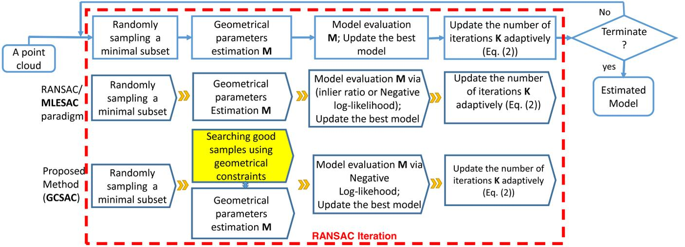
**Fig. 1.** Overviews of the proposed method (GCSAC) and the conventional RANSACs and a fitting scheme. Top panel: The original RANSAC/MLESAC paradigms; Bottom panel: Our proposed method, GCSAC.
