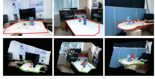
Fig. 5. Top line is some results of table plane detection step. The detected table planes are marked by the red color boundary; Bottom line is some results of table plane detection in the point clouds, table plane is marked by green color points (3-D contour), red color vector is the normal vector of the table plane.
